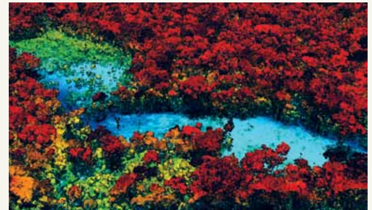
Figure 29: Laser-based measurements – LIDAR – assess forest biomass, creating 3-D profiles of forest down to individual trees (The Carnegie Institution for Science and WWF, in collaboration with the Peruvian Ministry of Environment (MINAM))
